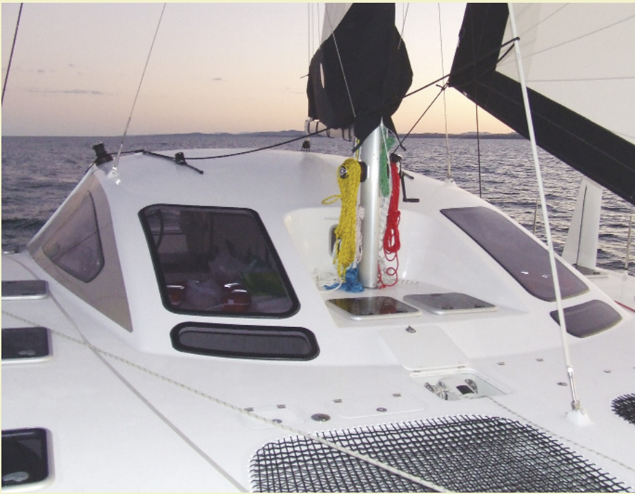
Note: Flat working area around the base of the mast.
