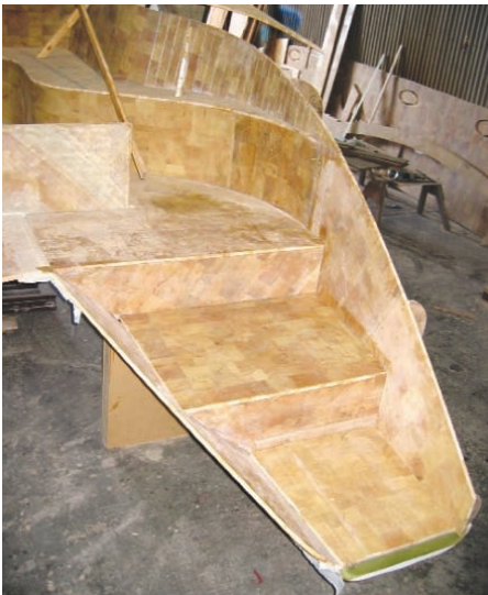
Aft steps and cockpit furniture assembled.
