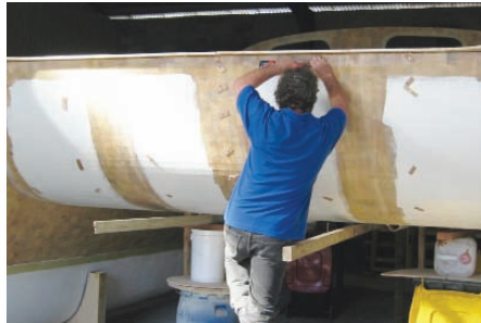
Fixing the curved section of the bridgedeck up in position.
