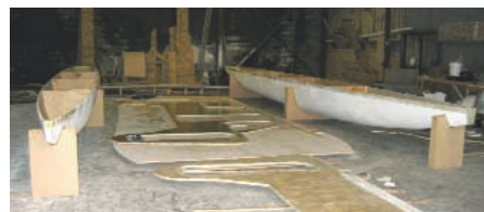
Both hulls ready for bulkheads to be fitted. Day one of assembly.
